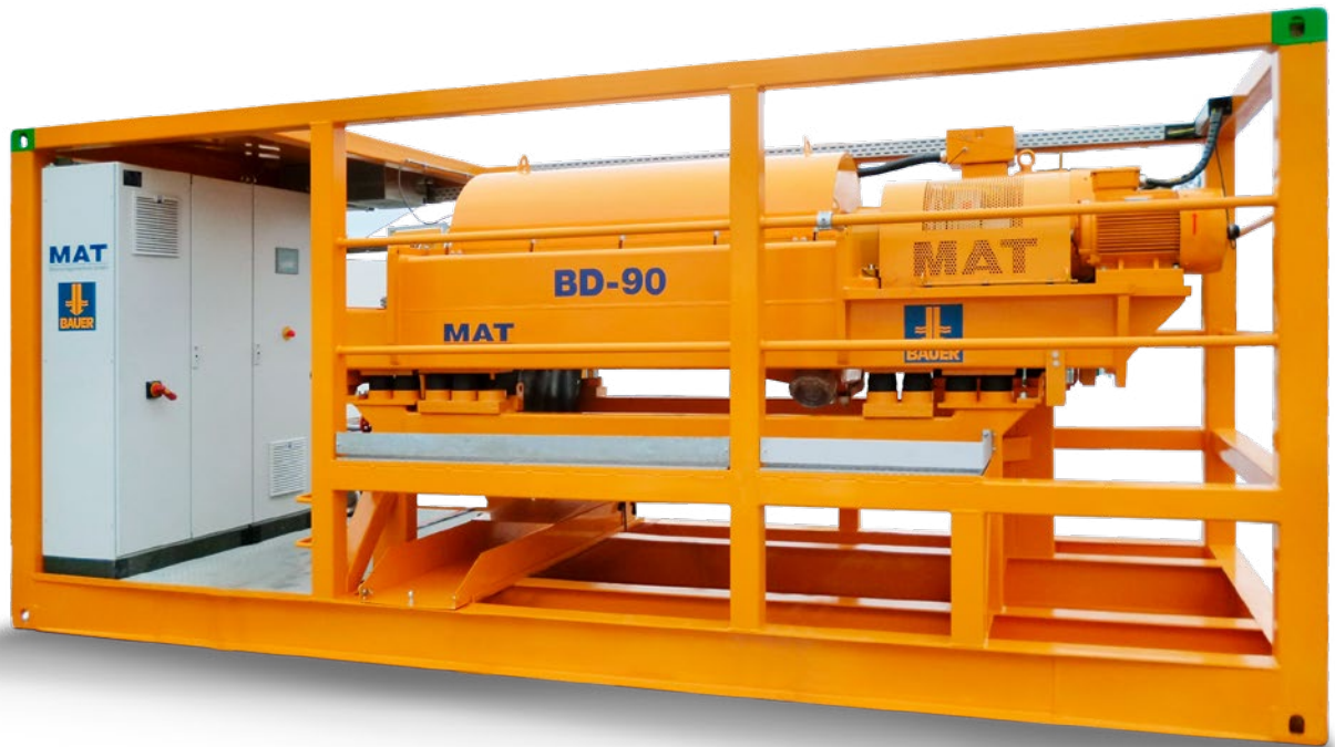
Decanter centrifuge BD-90 in open 20' container frame
